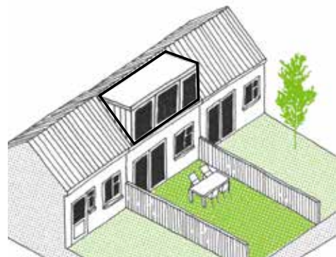
Avoid: an overbearing full-width box dormer to the rear slope of the house.
